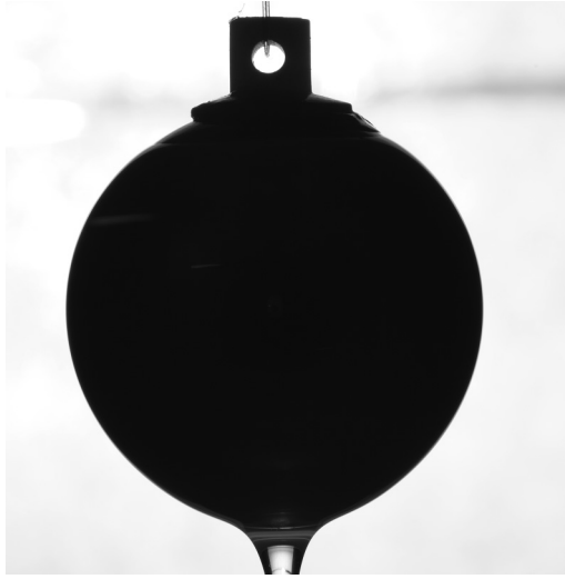
FIG. 6. Example snapshot of an alumina smooth particle coated in 1 Pa s silicone oil. The dripping process is exclusively gravity driven.
