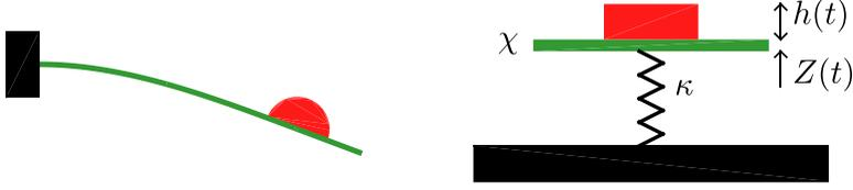
FIG. 14. Lumped-element model of the coupled vibration of a drop on a cantilever beam. (Left) The configuration investigated by Erfanul Alam and Dickerson [45]. (Right) The associated lumped-element model. The real drop is replaced by a cuboid drop of height  $h(t)$ . The beam is replaced by a rigid board (proof mass) of mass  $\chi$  at vertical position  $Z(t)$  supported by a spring of stiffness  $\kappa$ . All variables in the lumped-element model are dimensionless.
