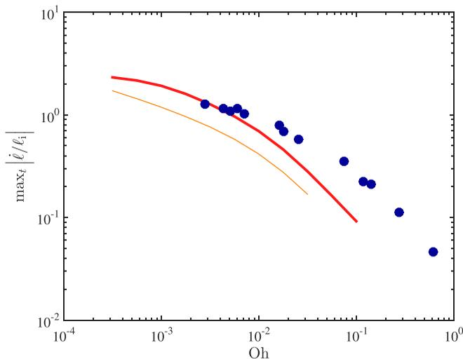
FIG. 9. Maximum retraction rate  $|\dot{\ell}/\ell_i|$  experienced by a sessile drop, as a function of Oh, for  $\text{Bo}_z = -0.6$ ,  $\gamma = 0.17$  and  $\zeta = 0.01$ . The dots correspond to measurements from Bartolo *et al.* [38] (with  $\text{Bo}_z \in [-0.72, -0.45]$  and initial normalized spreading diameter between 6 and 10). The thick red line (respectively, thin orange line) corresponds to numerical simulations of cuboid drops with  $\ell_i = 6$  (respectively,  $\ell_i = 10$ ).
