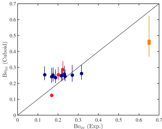
FIG. 12. Parity plot of the critical Bond number  $Bo_{xc}$  for the cuboid drop vs experiments from Podgorski *et al.* [40] and Podgorski [41] (dark blue dots), Le Grand *et al.* [42] (red dots), and original measurements reported in Supplemental Material [30] (orange dots). The error bars correspond to  $\lambda_w \in [-\zeta, \zeta]$  in the cuboid model [Eqs. (40) and (42)] and the dots are in  $\lambda_w = 0$ . The black line is the bisector of the first quadrant.
