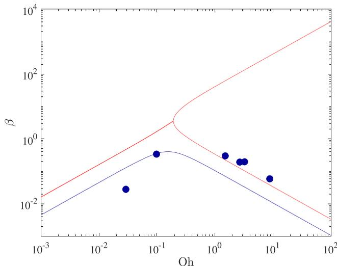
FIG. 15. Decay rates  $\beta_1$  (dark blue) and  $\beta_2$  (red) of the vibration modes associated to the cuboid drop on mass-spring system, as a function of the Ohnesorge number  $\text{Oh}$ , for  $\chi = 2.1$  and  $\kappa = 160$ . The solid lines correspond to the cuboid drop while the dark blue dots correspond to values inferred from the data of Erfanul Alam and Dickerson [45], for their beam of intermediate thickness. The corresponding asymptotic regimes are given in Table II.
