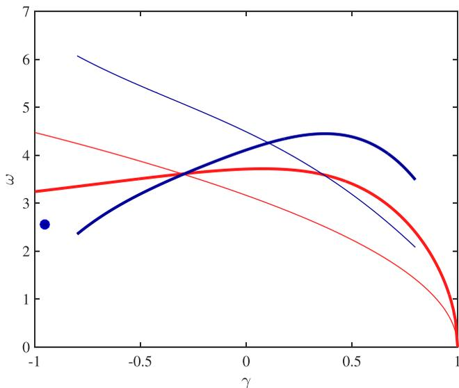
FIG. 5. Variation of the natural frequency  $\omega$  of a sessile drop with  $\gamma$ , for  $Bo_z = 0$ . Red lines correspond to cuboid drops, while dark blue lines correspond to the numerical solution of Zhang *et al.* [35] for real drops. Thick lines represent the zonal (2,0) mode, while thin lines represent the sectoral (2,2) mode. The dark blue dot corresponds to the experimental data from Mettu and Chaudhury [36].
