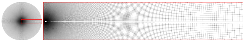
FIG. 12. Left: Mesh nodes for the full domain. Right: Zoomed view of the downstream domain sector.
