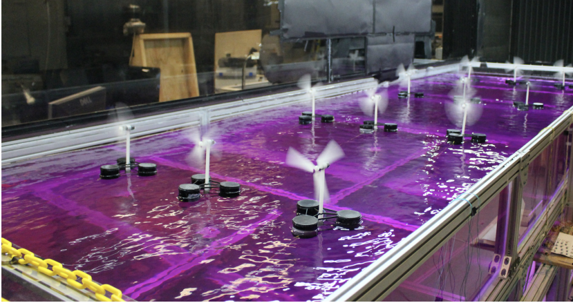
FIG. 1. Photograph of the scaled floating wind farm setup in the Portland State University wind and water tunnel.
