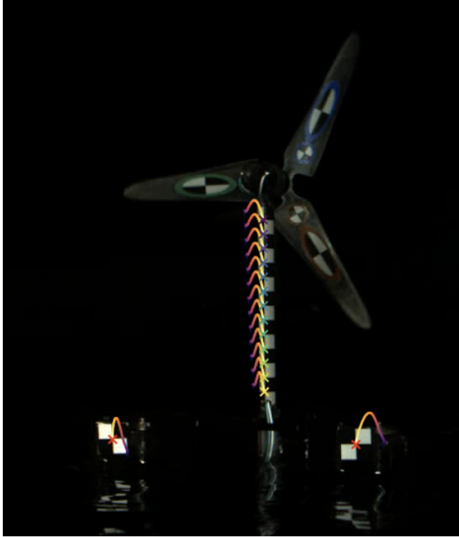
FIG. 4. Camera snapshot used for optical tracking, with indication of tracked markers and their previous trajectory for an incoming hub wind speed of 2.9 m/s and 1.2 Hz wave conditions.
