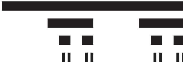
FIG. 1. Demonstration of how a fractal set of box-counting dimension 1/2 is formed. At every step (down) the initial set is split into four equal subsets out of which subsets 1 and 3 are disregarded. After N steps there are n = 2^N sets left of length \ell = L/4^N . Therefore the number of “boxes” of length \ell required to cover the remaining sets are n = (L/\ell)^D with D = 1/2 .
