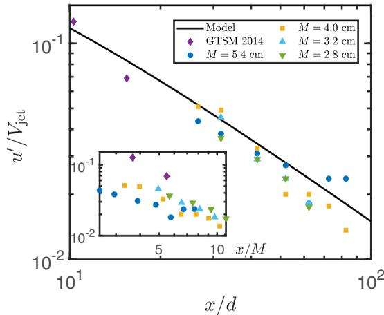
FIG. 9. The decay of turbulent velocity fluctuations as a function of the axial location normalized by  $d$  or  $M$  (inset). Data presented in this figure are the same as those described in Fig. 8. The black solid line is obtained from Eq. (6).
