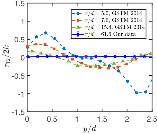
FIG. 6. One component of the Reynolds stress at four different axial locations downstream of a jet array. The three near-field measurements ( $x/d \leq 15$ ) were from the work by Ghahremanian *et al.* [44] (GSTM 2014) and the remaining far-field result ( $x/d \gg 15$ ) was acquired from Experiment I.4 using Array 1 at  $x = 5.7M$ .
