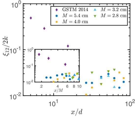
FIG. 8. The decay of the spatial variation of the Reynolds stress as a function of the normalized axial location. Purple diamonds represent the near-field data from the work by Ghahremanian *et al.* [44] (GSTM 2014), and other markers represent our data from Experiment I.1–I.4 using different jet spacings  $M$ .
