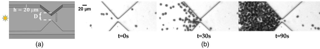
FIG. 1. (a) Schematic of bottleneck-shaped microchannel of thickness  $20\text{-}\mu\text{m} \sim 2 \times$  diameter of CR. The dashed rectangle represents the zone over which time lapses are measured. A light source is placed on the left, triggering a left to right swimming motion. (b) Snapshots of the jamming process through a  $D = 10\text{-}\mu\text{m}$  constriction at different times.
