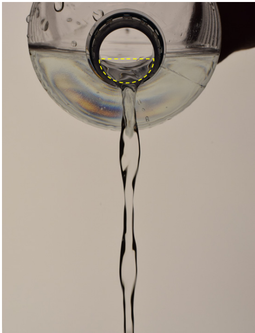
FIG. 1. Pouring water from a bottle. (a) Chain oscillations are excited because the initial cross section is noncircular, as highlighted by the dashed line.
