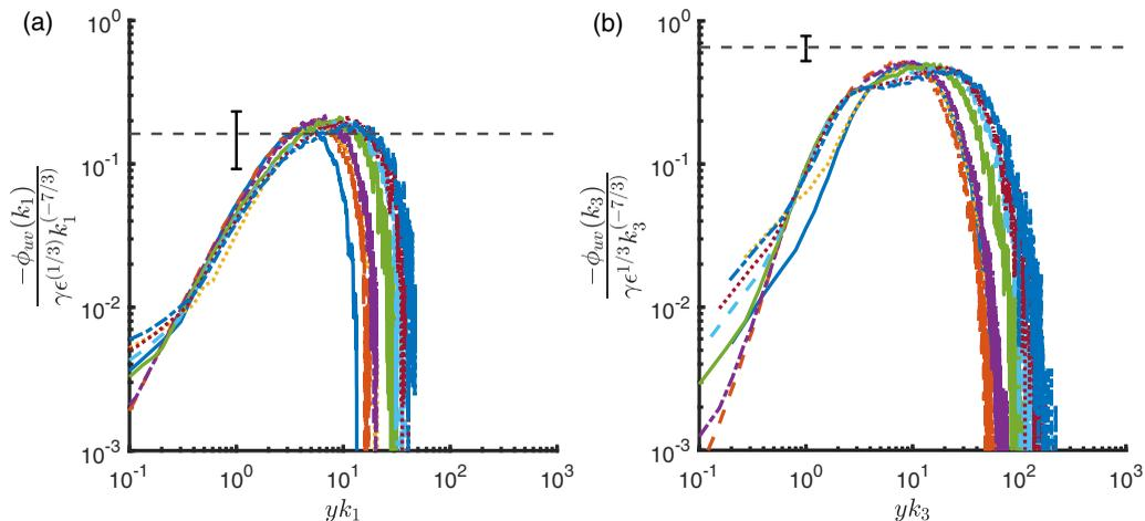
FIG. 3. (a) Compensated streamwise spectra and (b) compensated spanwise spectra for channel flow from the JHTDB. Lines have the same meanings as in Fig. 1.
