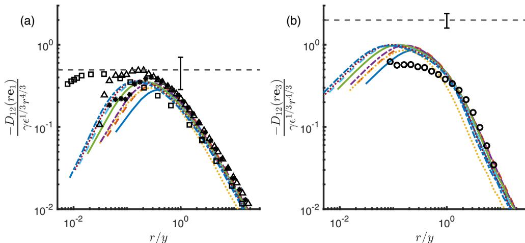
FIG. 2. (a) Compensated streamwise structure functions and (b) compensated spanwise structure functions. Lines and symbols are the same as in Fig. 1. The predicted inertial range behavior is marked by the dashed horizontal lines. The error bars are a result of the uncertainty in the prefactor.
