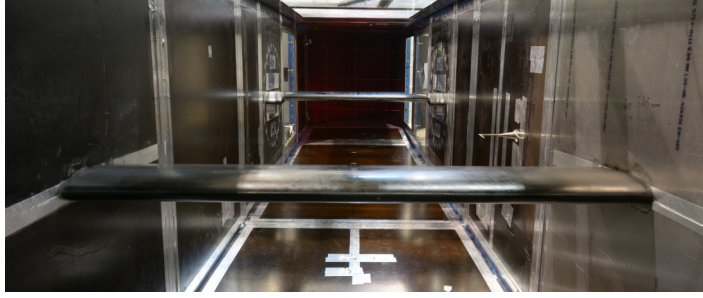
FIG. 1. Experimental setup inside the MUB test section showing the NACA-0021 gust generator airfoil (front), the hot wire probe, and the DLR-F15 research airfoil (back).
