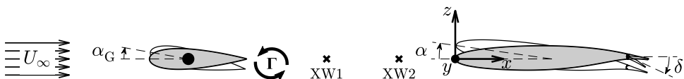
FIG. 2. Schematics of wind tunnel setup including the gust generator, the two X-wire positions XW1 ( x/c = -2.53 ) and XW2 ( x/c = 1.16 ), and the DLR-F15 research airfoil. Also shown are the gust generator angle of attack \alpha_G , the airfoil angle of attack \alpha , and the flap angle \delta . Not all dimensions are to scale.
