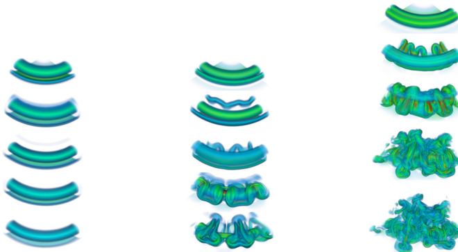
FIG. 24. Vorticity volume visualization at several instances of time for ring impact against a no-slip wall at \Lambda = 0.1 and white noise perturbations. Reynolds number increases from left to right ( \text{Re}_\Gamma = 1000 , \text{Re}_\Gamma = 2000 , and \text{Re}_\Gamma = 3500 ), and time increases from top to bottom ( t = 12, 18, 21, 23 , and 28 for left, 12, 16, 18, 21, 24 for center and 12, 15, 18, 21, 23 for right). Red denotes regions of particularly high vorticity, and blue denotes regions of low vorticity.
