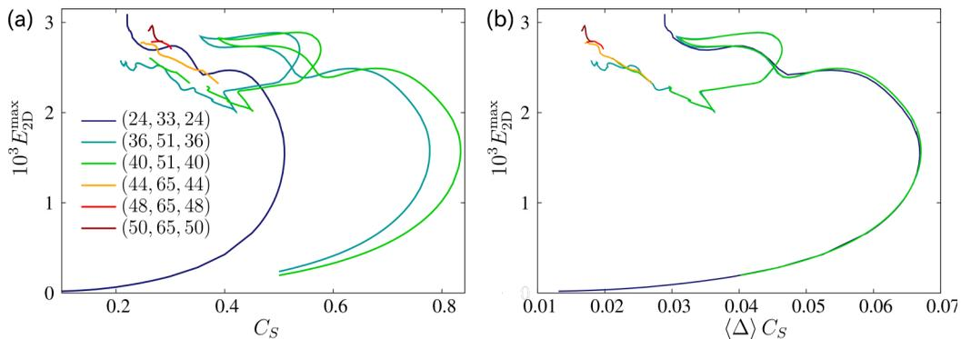
FIG. 4. Bifurcation diagram of the LES gentle and active UPOs at  $Re = 2000$ . The colored lines, from dark-blue to dark-red, represent the sets of the number of grid points from  $(N_1, N_2, N_3) = (24, 33, 24)$  to  $(50, 65, 50)$ , and so the filter widths.
