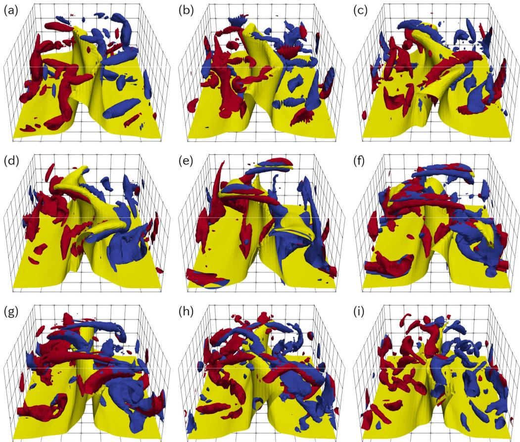
FIG. 9. Snapshots of the LES active UPO of the period  $T = 79.25$  at  $Re = 2000$  and  $\langle \Delta \rangle C_S = 0.01658$  [ $C_S = 0.2598$ ,  $(N_1, N_2, N_3) = (50, 65, 50)$ ,  $h^+ = 105$ ]. Time elapses from (a) to (i) by  $T/20$ . The definition of isosurfaces is the same as Fig. 5, but  $u_1 = 0.2$  ( $u^+ = 21.6$ ) and  $Q = 0.1$ .
