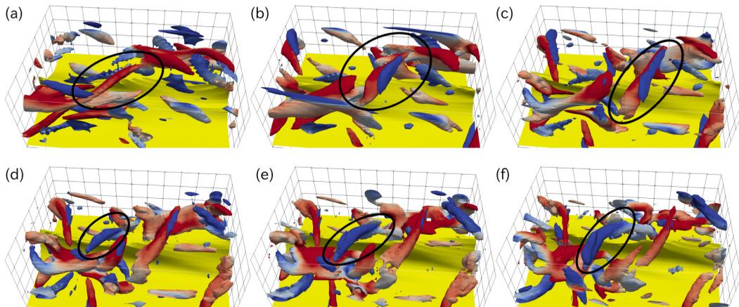
FIG. 10. Development of spanwise vortices. The yellow objects are the isosurfaces of the streamwise velocity  $u_1 = 0.3$ , while the blue to red objects denote  $Q = 0.1$  within the range of  $-0.75 \leq \omega_3 \leq 0.75$ . Time elapses from (a) to (c) by  $T/20$  ( $3T/20 \leq t \leq 5T/20$ ) and from (d) to (f) by  $T/40$  ( $55T/200 \leq t \leq 65T/200$ ). The black circles are used for emphasis on the spanwise vortices.
