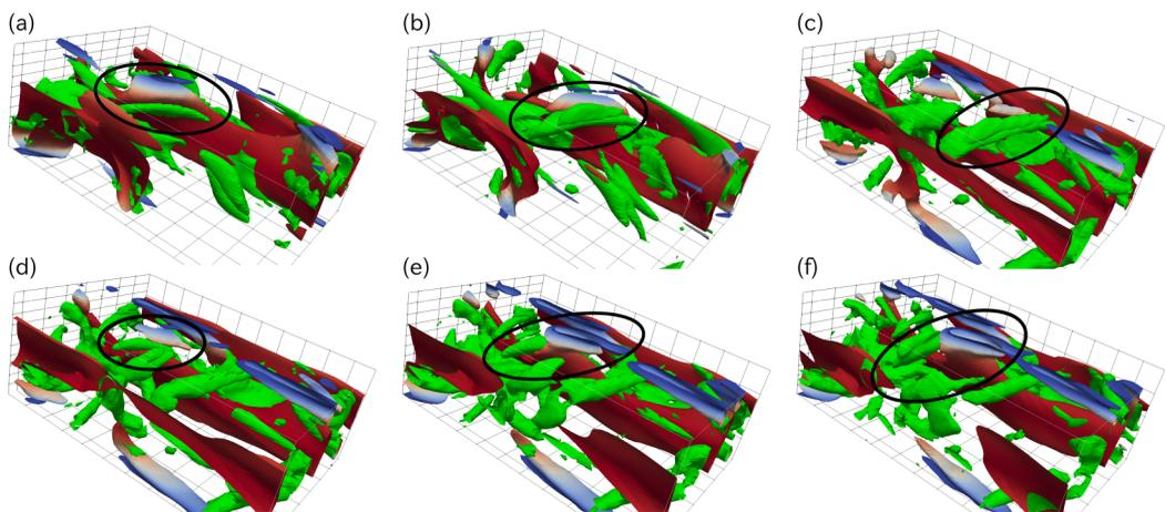
FIG. 11. Reynolds shear stress  $-u_1'u_2'$  of the LES active UPO. The blue to red objects indicate the isosurface  $|u_1'u_2'|/(\hat{u}_1\hat{u}_2) = 1.75$  where the color means the value of the Reynolds shear stress  $-u_1'u_2'$  from 0 to 0.014. The green surfaces indicate  $Q = 0.1$ . The time series of (a) to (c) and of (d) to (f) are the same as Fig. 10.
