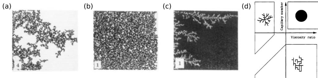
FIG. 3. Lenormand *et al.* [57] studied drainage in porous media and found that the fluid-fluid front can advance through (a) invasion percolation, (b) stable displacement, or (c) viscous fingering, depending on  $Ca$  and  $M$ . The character of displacement is synthesized in the (d) phase diagram of Lenormand *et al.* [57]. Adapted from Lenormand [58].
