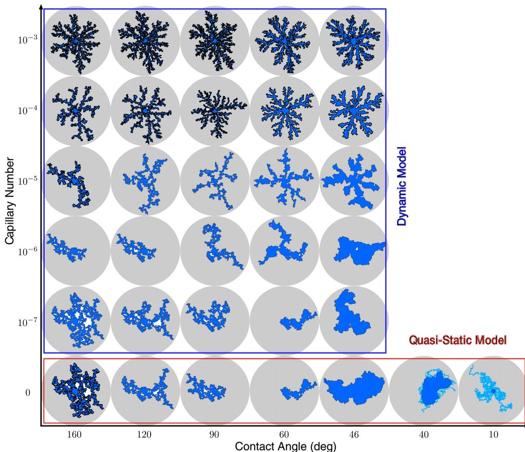
FIG. 6. Numerical simulation of fluid-fluid displacement under different  $Ca$  and wettability using quasi-static [72] and dynamic moving-capacitor [73] models. The simulations cover the majority of the  $Ca$ - $M$  parameter space along with the dominant flow regimes demonstrated in experiments (Fig. 4). Adapted from Primkulov *et al.* [73].
