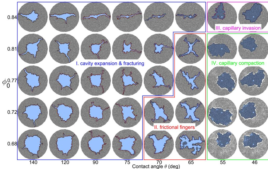
FIG. 13. Visual phase diagram of the invading fluid morphology at breakthrough corresponding to different substrate wettabilities (contact angle  $\theta$ ) and initial packing densities  $\phi_0$ . Four distinct morphological regimes are identified: (I) cavity expansion and fracturing, (II) frictional fingers, (III) capillary invasion, and (IV) capillary compaction. Reprinted from Meng *et al.* [161].
