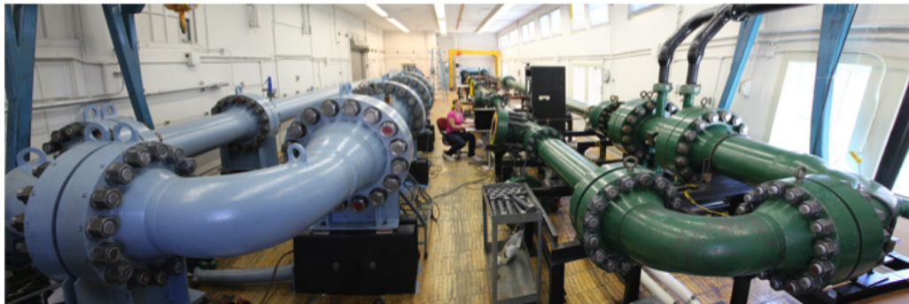
FIG. 3. Left: Princeton High Reynolds number Testing Facility (HRTF), completed 2007. Operating conditions: p = 1 to 200 bar (abs), D = 0.5 m dia., L = 3.6 m, V_m = 10 m/s, Re_m \approx 90 \times 10^6 /m. Right: Princeton Superpipe, completed 1994. Operating conditions: p = 1 to 200 bar (abs), D = 0.129 m dia., L = 22 m, V_m = 35 m/s, Re_m \approx 270 \times 10^6 /m. Reproduction with permission from D. Quinn.
