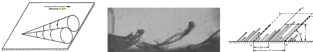
FIG. 9. Left: Townsend roller eddies. Reproduction with permission from [29]. Middle: Theodorsen hairpin eddies. Reproduction with permission from [42]. Right: Perry and Chong's wall-attached eddies. Reproduction with permission from [30].
