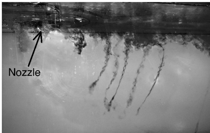
FIG. 6. Flow visualization of the Fric and Roshko vortices.
