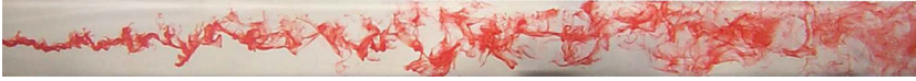
FIG. 2. Dye visualization of the plume at Re = 10\,000 with a nozzle diameter of 4.7 mm.
