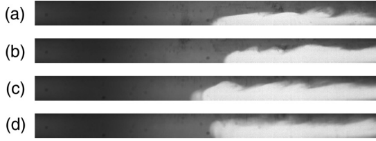
FIG. 3. Front shape images at \beta = 75^\circ , \hat{v} = 1 \text{ mm}^2/\text{s} , and At = 10^{-2} , with increasing rotation speed (a)–(d): \hat{\omega} = 0, 1.05, 2.09 , and 3.14 \text{ rad/s} . The photos are captured at \hat{t} = [7.4, 8.6, 10.3, 13.0] \text{ s} from top to bottom. The field of view is 19 \times 240 \text{ mm}^2 , 45 mm below the gate valve. The side view of the flow is shown here and throughout the paper, unless otherwise stated.
