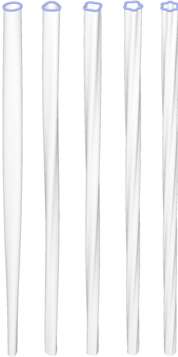
FIG. 14. Twisted jets with n -trigonometric cross sections. n = 2, 3, 4, 5, and 6 , from left to right. The jet length L_z = 77 r_0 and the nondimensional amplitude \delta = 0.1 are all the same.
