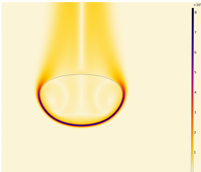
FIG. 7. Temperature gradient ( K/m ) in and around the drop for our reference simulation no. 4 in Table II at time t^* = 0.055 .
