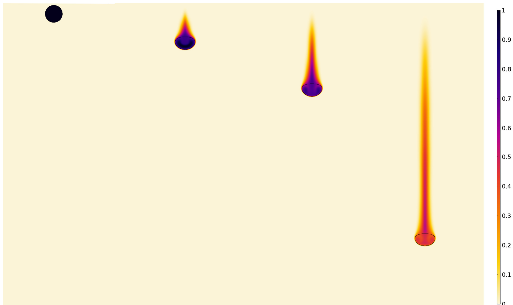
FIG. 3. Dynamical and thermal evolutions of the metal drop as a function of time for simulation no. 4 in Table II. The color presents the temperature anomaly normalized by its initial value T^* . The black solid line separates the metallic material from the magma ocean. From left to right, the time normalized by the thermal diffusion time is t^* = 0, 0.01, 0.02, \text{ and } 0.05 .
