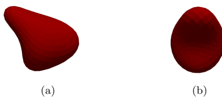
FIG. 3. Unconfined flow with \nu = 0.90 , C_a = 4 , \lambda = 1 . Tank treading slipper. (a) Side view of slipper and (b) Rear view of slipper.
