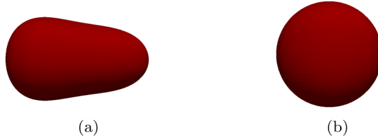
FIG. 14. Confined flow: bell shape with \nu = 0.90 , \lambda = 1 , C_n = 0.5 , C_a = 0.5 . (a) Side view and (b) Rear view.
