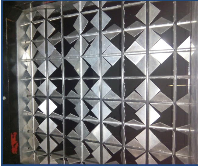
FIG. 1. Picture of the active grid used on the present work.
