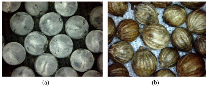
FIG. 3. Photos of the particles used in this investigation as granular matter: (a) glass beads, 2.0 mm mean diameter; (b) mustard seeds, 2.2 mm mean diameter.
