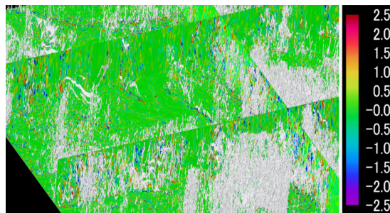
FIG. 8. Distributions of the horizontally oriented vorticity (color contour) at three vertical walls whose top view coordinates are indicated by black dashed lines in Fig. 6(a) together with the color contour at the bottom plane at z = 0 for N4096- \lambda 64 . The enstrophy is also plotted by the white 3D isosurface. The threshold of the white isosurface was set at m + 3\sigma , where m and \sigma are the mean and standard deviation, respectively. The vertical real-space scale is doubled. For vorticity, calm regions are colored green in the planes, and active regions are colored red or blue (as in the color scale bar). Large structures (SOVs) consist of a mass of assembled tiny active spots and specks with sizes comparable to or smaller than the CLS. The bottom plane cross section corresponds to the cross section illustrated in Fig. 6(b) and the active SOV structure has one-to-one correspondence. See also Movie S2 [26] for a temporal evolution of the structures.
