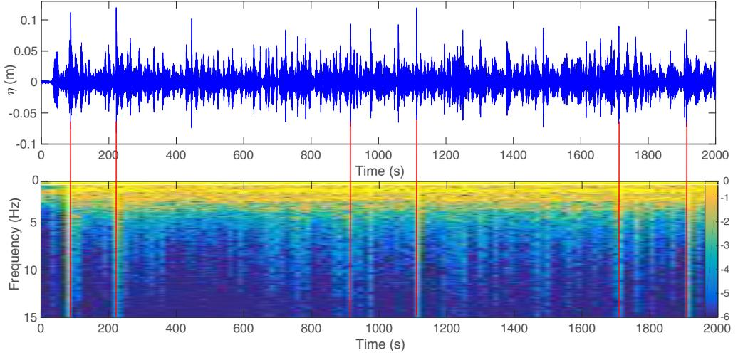
FIG. 9. Top: Temporal wave height signal for  $\tau = 0.44$  ( $\epsilon_\eta = 0.08$ ,  $\Delta f = 0.16$  Hz).  $x = 29.8$  m. Bottom: Time-frequency spectrum  $S_\eta(f, t)$  of the corresponding wave height  $\eta(t)$ . The color bar is a logarithmic scale of the spectrum amplitude. Large amplitude events of the wave signal correspond to maxima of the spectrum at high frequencies (see solid lines).
