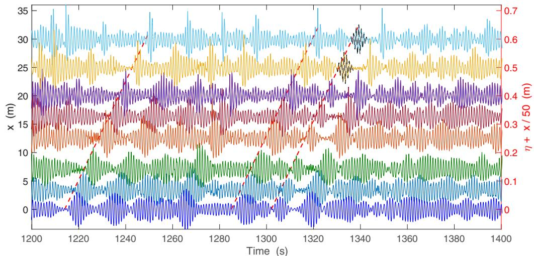
FIG. 3. Experimental evolution along the basin length  $x$  of the wave height  $\eta(t)$  recorded at different probe locations (from bottom to top:  $x = 0, 3.4, 7, 12.6, 16.3, 20.1, 24.9,$  and  $29.8$  m).  $\tau = 0.44$  ( $\epsilon_\eta = 0.08$  and  $\Delta f = 0.16$  Hz). Dashed (red) lines have a slope corresponding to the group velocity  $c_g$ . The dashed (black) line on top of the two upper curves is the theoretical shape of the envelope soliton of Eq. (8).
