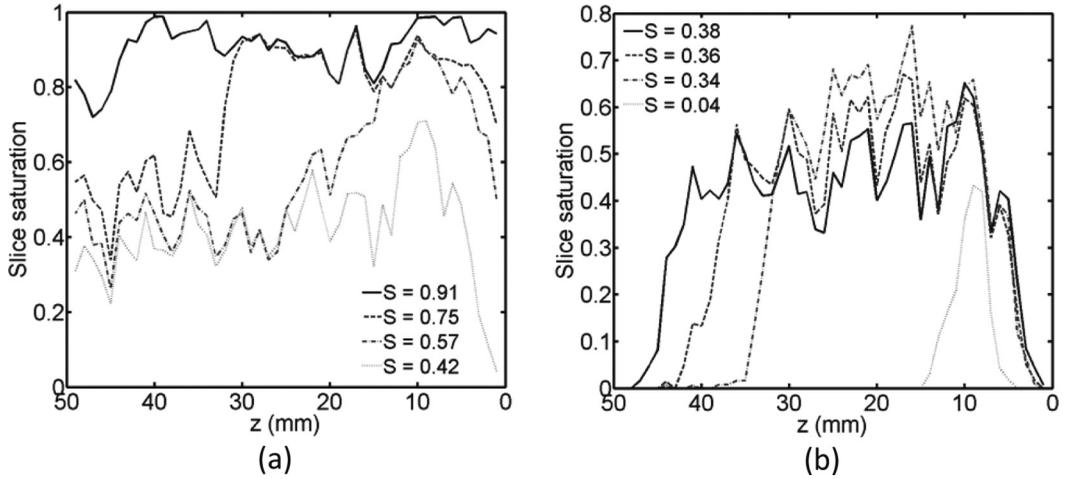
FIG. 8. Drying experiments: horizontal slice averaged saturation profiles computed from the phase distributions shown in Fig. 2. The top row corresponds to  $z = 0$  mm. (a) Periods 1 and 2 up to the full fragmentation of the liquid phase. (b) Periods 3 and 4, i.e., shrinking two-phase zone. Notice the increase in slice saturation between  $z \cong 8$  and 38 mm.
