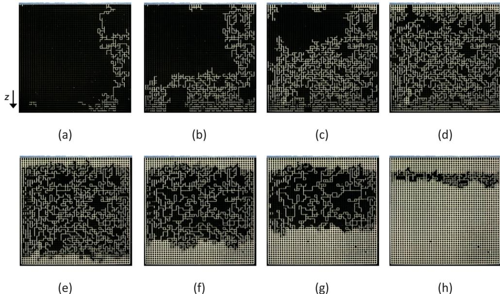
FIG. 2. Experimental phase distributions obtained from drying with  $dT/dz = 0.44 \text{ K mm}^{-1}$  and  $\bar{T}_{z=0} \cong 24^\circ\text{C}$ . Liquid and solid in black, gas phase in light gray. Vapor escapes from top edge. Shown are the snapshots for overall network saturation  $S = [0.91, 0.75, 0.57, 0.42, 0.38, 0.36, 0.34, 0.04]$ , from (a) to (h), respectively.
