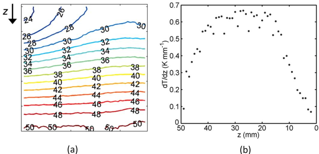
FIG. 1. (a) Temperature field with positive temperature gradient  $dT/dz$  imposed on the micromodel in the  $z$  direction.  $\bar{T}_{z=0} = 24^\circ\text{C}$  (top edge) and  $\bar{T}_{z=49L} = 50^\circ\text{C}$  (bottom edge). (b) The temperature contour lines indicate nonlinearity of the temperature gradient in the  $z$  direction.
