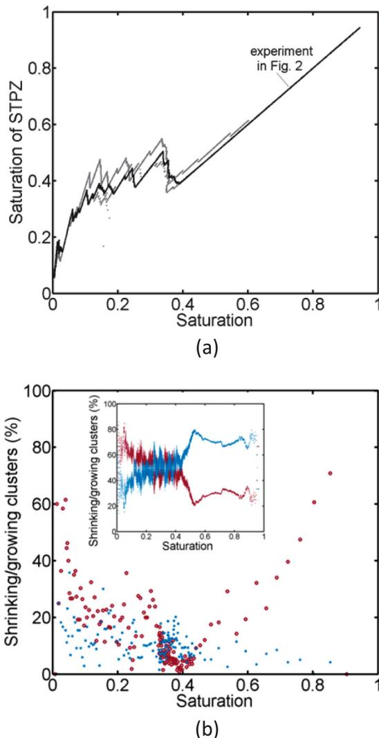
FIG. 12. (a) Saturation of the STPZ (experiment from Fig. 2 in black; additional experimental curves in gray). (b) Percentage ratio of shrinking (in red) and growing (in blue) clusters related to the current total number of clusters determined by image processing of experimental patterns (see text); the inset shows the same type of data from the PNM simulations (see text).
