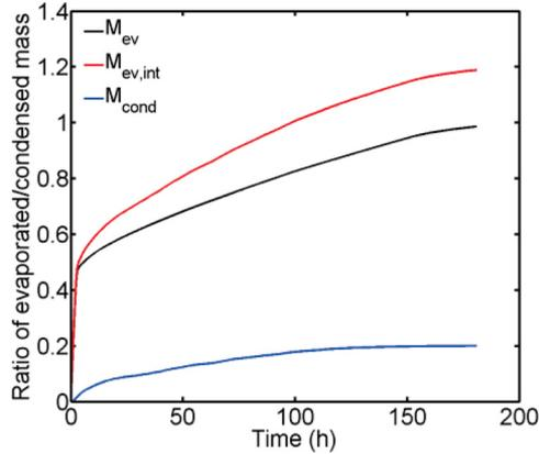
FIG. 13. PNM computation of the variation of  $M_{ev}(t)$  (net evaporation),  $M_{ev,int}(t)$ , and  $M_{co}(t)$  [Eq. (21)] related to the initial mass of water in the PN [ $M(t=0) = 0.0284$  g].
