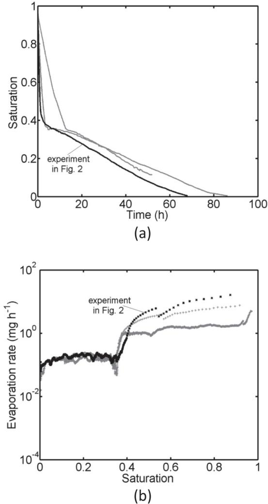
FIG. 6. Drying experiments: (a) drying curves and (b) drying rates in a semilogarithmic plot. The curves corresponding to the experiment discussed above and presented in Fig. 2 are shown in black color; experiments from Figs. 4(b) and 4(c) are shown in gray.
