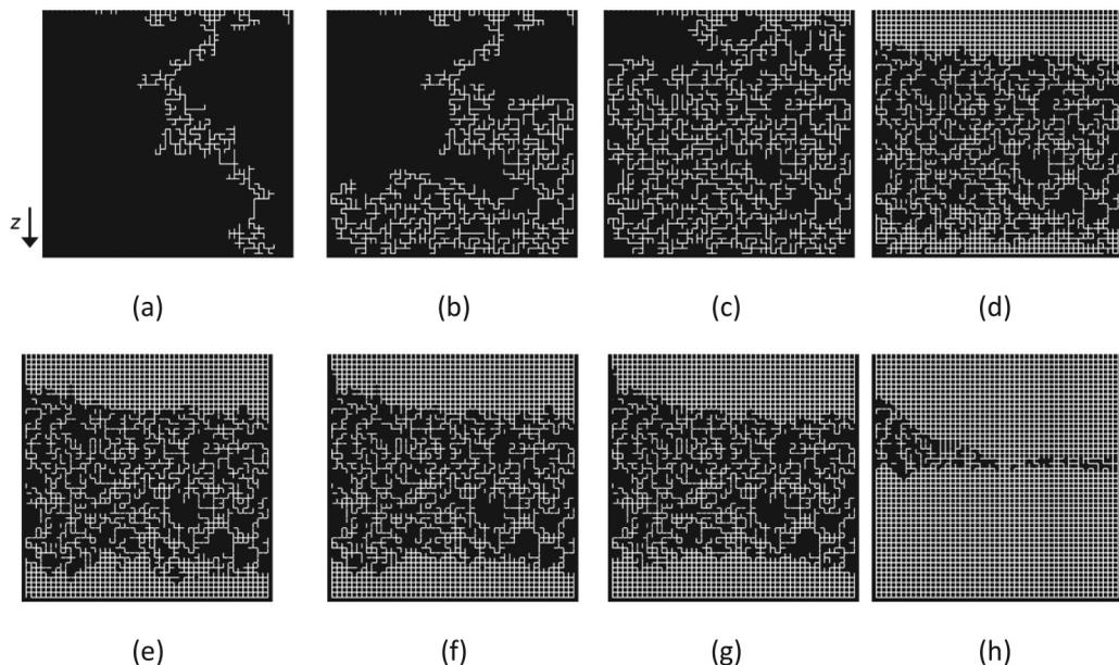
FIG. 3. PNM computed phase distributions obtained from drying with the same temperature setting as in Fig. 2. Liquid and solid in black, gas phase in white. Vapor escapes from top edge.  $S = [0.91, 0.75, 0.57, 0.42, 0.38, 0.36, 0.34, 0.04]$ , from (a) to (h), respectively.
