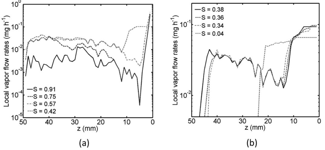
FIG. 9. PNM simulations: total through-plane vapor flow rates from the simulation corresponding to Fig. 3. The top row is located at  $z = 0$  mm. Curves computed for various overall network saturation (a)  $S = [0.91, 0.75, 0.57, 0.42]$  and (b)  $S = [0.38, 0.36, 0.34, 0.04]$ .
