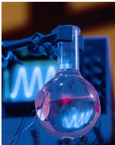
FIG. 1. Setup for single-bubble sonoluminescence. Piezoelectric transducers are glued to a flask filled with water. They excite a standing acoustic wave in which the light-emitting bubble is trapped. The photo was taken by Rüdiger Toegel, Physics of Fluids, Twente, 2000.
