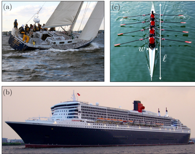
FIG. 1. Pictures of (a) a 44-ft sailing boat: length-to-width aspect ratio 3 and typical Froude number 0.6, (b) the Queen Mary 2 liner: length-to-width aspect ratio 8.4 and typical Froude number 0.26, and (c) a coxless quadruple scull rowing boat: length-to-width aspect ratio 31 and typical Froude number 0.54. See Table I for details and characteristics of other boats.
