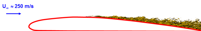
FIG. 8. Sketch of the flow over an airfoil at low angle of attack emphasizing the TBL in the APG region on the suction side.
