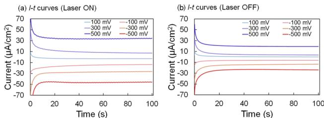
FIG. 5. Response of Au-PVP nanofluid to applied bias voltages shown as current  $I$  vs time  $t$  curves in the (a) presence and (b) absence of the laser beam in a two-electrode setup; the working electrode is a silver wire and the counter or reference electrode is a silver flag. The intensity of the laser is 440 mW and it travels at a depth of 2.2 mm from the free surface. The distance between the electrodes is kept constant.
