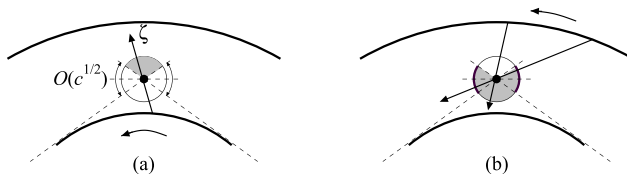
FIG. 3. Schematics of trajectories of collisionless molecules and the range of the direction of the molecular velocities arriving from the rotating cylinder. (a) Inner rotation and (b) outer rotation. The shaded area represents the directional range of molecular velocities arriving from the rotating cylinder. The thick arc in panel (b) indicates the directional range of the molecular velocities traveling from the outer cylinder to the outer cylinder, which is of O(\sqrt{c}) .
