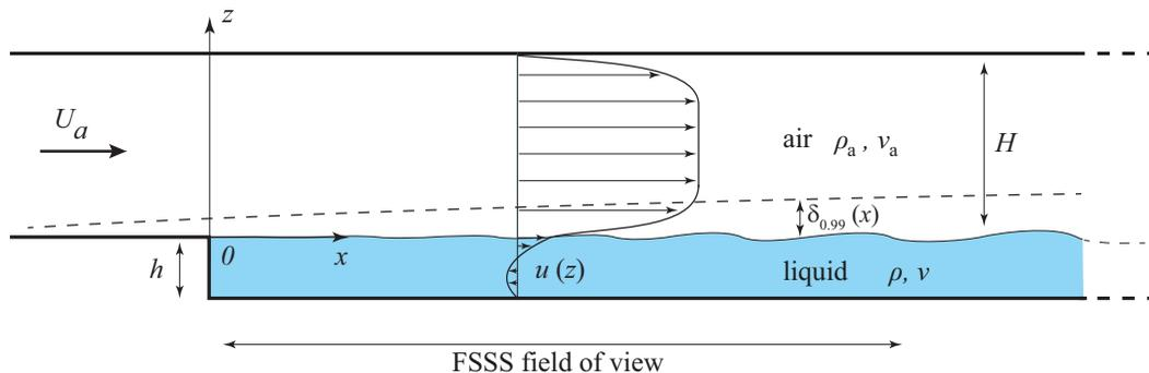
FIG. 1. Sketch of the system. The velocity profiles in the air and in the liquid are not drawn to scale: The air velocity is typically 100 times larger than the liquid velocity. The wave amplitude is exaggerated.
