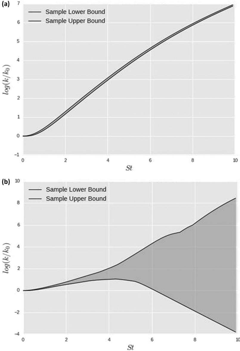
FIG. 3. Sample prediction intervals for an initially isotropic Reynolds stress at  $\frac{Sk}{\epsilon} = 27$ . (a) Axisymmetric contraction. (b) Axisymmetric expansion.
