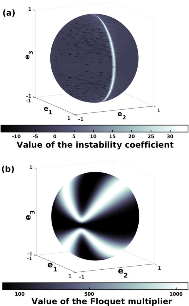
FIG. 7. Contours exhibiting the relationship between modal alignment in unit wave number space and modal stability for representative cases of (a) hyperbolic flow and (b) elliptic flow.
