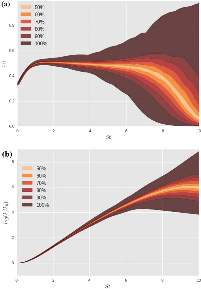
FIG. 4. Sample prediction intervals at different levels of certitude for the (a) Reynolds stress anisotropy ( $r_{22} = \frac{K_{22}}{k}$ ) and (b) turbulent kinetic energy,  $k$ , for a plane strain mean flow (initially isotropic Reynolds stress at  $\frac{Sk}{\epsilon} = 27$ ).
