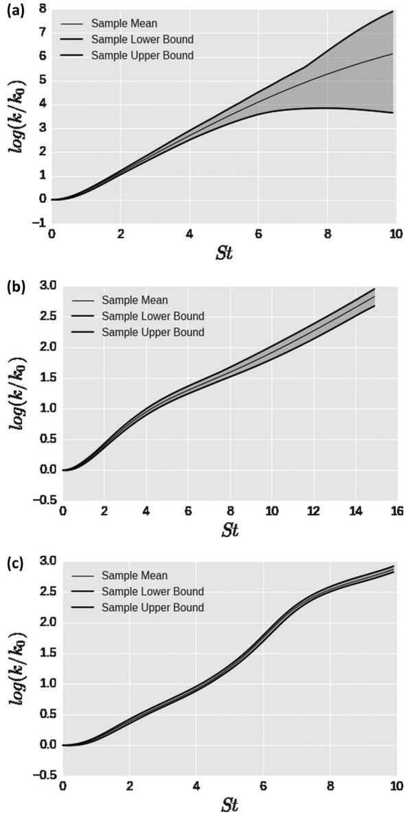
FIG. 2. Sample prediction intervals for an initially isotropic Reynolds stress at  $\frac{Sk}{\epsilon} = 27$ . (a) Hyperbolic flow. (b) Planar pure shear. (c) Elliptic flow.
