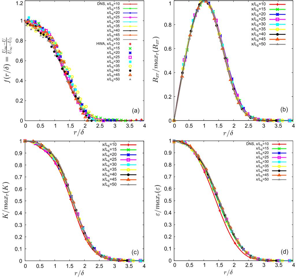
FIG. 1. Mean flow profiles at different streamwise distances plotted using similarity scalings (a). Markers stand for HWA measurements while lines stand for DNS data. Profiles of  $R_{xr}$  (b),  $K$  (c), and  $\varepsilon$  (d) normalized by the maximum radial value at different streamwise distances versus  $r/\delta$  for DNS only.
