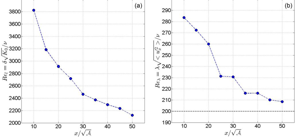
FIG. 2. Streamwise variation of local Reynolds number  $Re_L = \sqrt{K_0} \delta / \nu$  (a). Streamwise variation of Reynolds number  $Re_\lambda = \sqrt{\langle u_x^2 \rangle} \lambda / \nu$  based on the Taylor microscale  $\lambda = \sqrt{15 \nu \langle u_x^2 \rangle / \varepsilon_{\text{iso}}}$  (b). The black dashed line represents the lower limit  $Re_\lambda = 200$  for nonequilibrium scalings proposed in Ref. [5].
