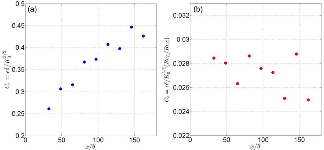
FIG. 3. Equilibrium dissipation coefficient  $C_\varepsilon^{\text{Eq}} = \varepsilon_0 \delta / K_0^{3/2}$  (a). Nonequilibrium dissipation coefficient  $C_\varepsilon^{\text{Noneq}} = \varepsilon_0 \delta / K_0^{3/2} (Re_L / Re_G)^{3/2}$  (b).
