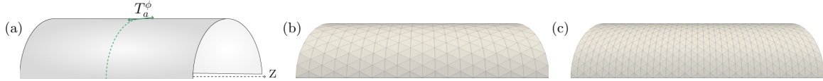
FIG. 4. (a) We consider a local increase in active in-plane surface stress of a cylindrical membrane. (b), (c) Membrane meshes as in main text with two different resolutions, (a) \Delta z = 0.2 , \Delta\phi = 0.2 and (b) \Delta z = 0.1 , \Delta\phi = 0.15 , respectively.
