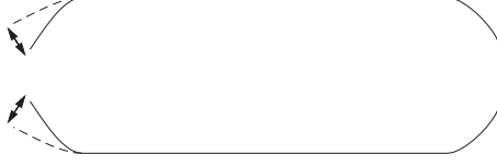
FIG. 4. Sketch of a body motion for which the kinetic friction model has no solution, so a model of static friction is used.
