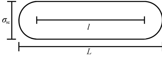
FIG. 1. Sketch of a spherocylinder in two dimensions. It consists of a rectangle and two half circles. A spherocylinder is described by its length L , the line segment l , and its diameter \sigma_{sc} .
