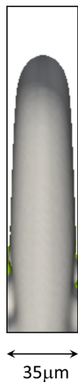
FIG. 3. Side view of the numerical domain ( 35 \mu\text{m} in thickness) showing one of the two oscillating fingers intersected by the yz plane that passes through its tip. The tip radius of curvature is roughly equal to 11.5 \mu\text{m} here.
