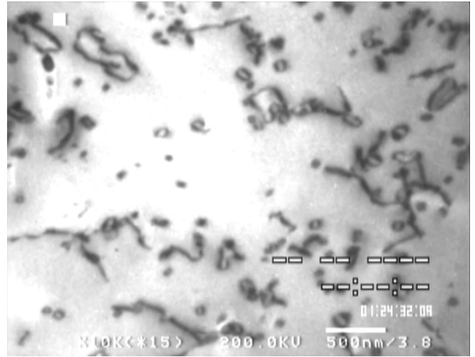
FIG. 1. TEM snapshot of in situ annealing of ion-irradiated tungsten (2-MeV W^+ ions, 500^\circ\text{C} , 10^{14} W^+/\text{cm}^2 ) at 700^\circ\text{C} . Adapted with permission from [2].
