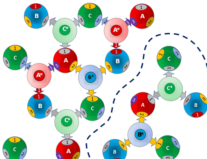
FIG. 6. Schematic representation of the reduced-set, nonrobust design. It contains N = 6 particle types, and K = 8 bond types. Note that both stacking configurations are possible for B^* and C^* particles, but only one will eventually be selected (after rearrangements) due to the presence of A^* .
