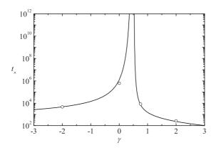
FIG. 3. Relaxation time  $t_{\times}$  vs the exponent  $\gamma$  for power-law expansions. The line represents the theoretical value obtained by solving the equation  $S(t_{\times}) = S_{\infty} + 0.05$  with S(t) and  $S_{\infty}$  respectively given by Eqs. (29) and (32). The symbols represent simulation results. The chosen parameters are  $t_0 = 1000$ ,  $c_0 = 1/100$ , and D = 1/2.
