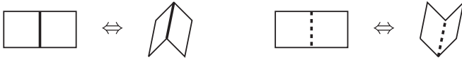
FIG. 1. Mapping of mountain folds to solid lines (left) and valley folds to dashed lines (right).
