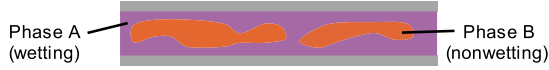
FIG. 1. Diagram showing the thin film morphology with layers of the wetting phase adjacent to the top and bottom substrates, and internal domains of the nonwetting phase.
