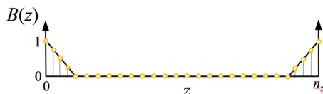
FIG. 2. Schematic of the B(z) function described in Eq. (6) used to induce preferential wetting on the top and bottom z boundaries.
