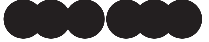
FIG. 2. Two-dimensional illustration when spheres become (vertical) disks. Each disk represents the excluded region, so its radius is twice larger than the radius of diffusing and absorbing particles. The center of the new disk must go through the channel between two central disks and it must reach the bottleneck (the horizontal segment).
