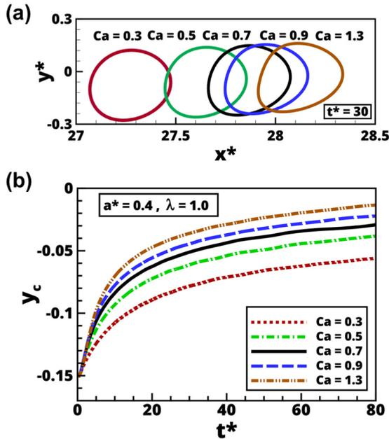
FIG. 7. The effect of varying  $Ca$  ( $Ca = 0.3$  to  $1.3$ ) on the migration of a drop initially placed at  $y_c = -0.15$ . (a) Drop velocity versus time. (b) Lateral position of the drop versus time. The other parameters are  $a^* = 0.4$  and  $\lambda = 1$ .
