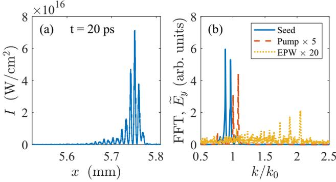
FIG. 4. PIC simulation of a DFBRAs as in Fig. 3 but with an initial phase difference of  $\pi$ . The spectra (b) of the amplified seed (solid blue), pump (dashed red), and EPW (dotted yellow) is similar to that without initial phase difference (Fig. 3) but the intensity of the amplified pulse (a) has a maximum at the center of the beat-wave envelope.
