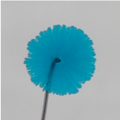
FIG. 8. Pattern formed by injecting a 400 mM CPCl solution at Q = 100 ml/h into caprylic acid (taken at t = 8 s).
