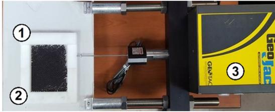
FIG. 7. Shear apparatus: 1, sliding portion of the shear box; 2, fixed portion of the shear box; and 3, load cell.
