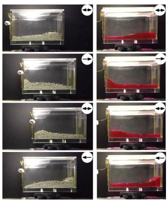
FIG. 3. Direct comparison of the liquidlike sloshing state (five layers of spheres with d = 2 mm at  $\Gamma \approx 0.80$ ) with the sloshing dynamics of a liquid (A = 7 mm, f = 1.7 Hz). As in Fig. 2, snapshots are taken at about  $0, \frac{1}{4}, \frac{1}{2}, \frac{3}{4}$  of the driving period, where the phase 0 is defined as the maximum leftward displacement.
