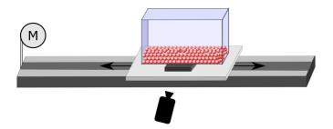
FIG. 1. Sketch of the experimental setup. A rectangular container is partly filled with monodisperse steel spheres and mounted on a sledge. The sledge is harmonically driven by a step motor with a frequency of 3 Hz, while the amplitude is varied to change the acceleration. The dynamics of the spheres is monitored by a camera from the front. In most of the measurements the diameter of the spheres is 4 mm.
