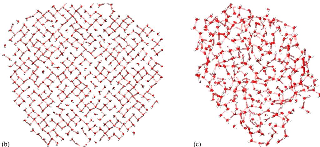
FIG. 7. (a) Number of hydrogen bonding at the interface of Au (100) and graphene in the last 500 ps of the simulation, Snapshots of water molecules at the interface of (b) Au (100), and (c) graphene.
