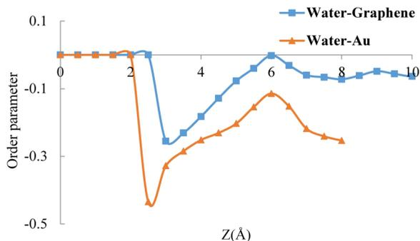
FIG. 6. Order parameter of water molecules along the Z axis.
