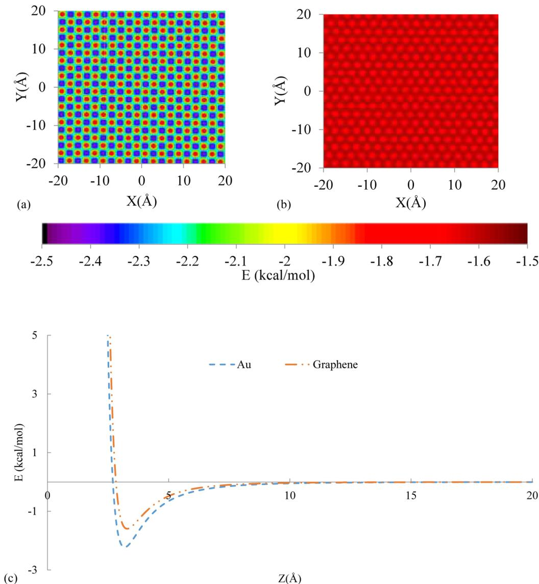
FIG. 3. Comparison of the contour map energy between one water molecule with (a) Au (100), and (b) graphene substrate. (c) Comparison of the interaction energy between a water molecule with Au (100) and graphene substrates along the Z axis.
