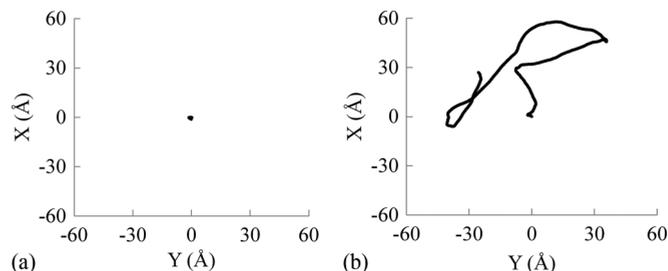
FIG. 9. Variations of center of mass of water molecules on (a) gold, and (b) graphene surfaces.
