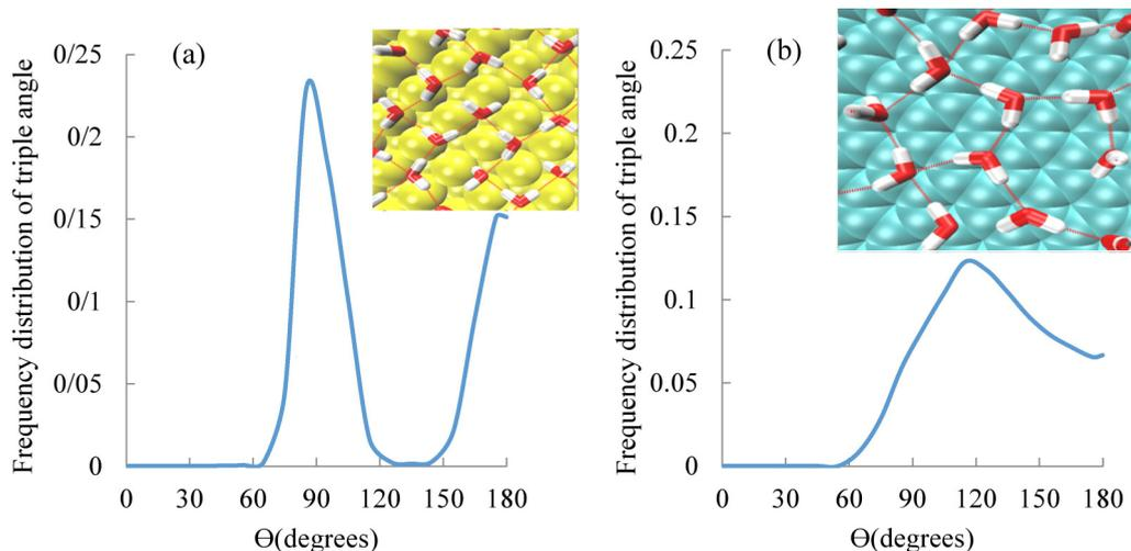
FIG. 4. Distribution of the triple angle between water molecules on the interface of (a) Au (100), and (b) graphene.
