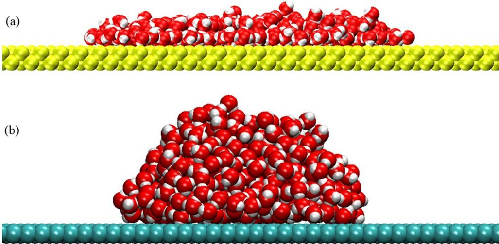
FIG. 1. The final snapshots of the water nanodroplet on (a) Au (100), and (b) graphene surfaces. Red, white, yellow, and green represent oxygen, hydrogen, gold, and carbon, respectively.
