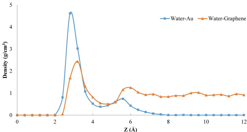
FIG. 2. Density profile of water molecules on Au (100) and graphene substrates.
