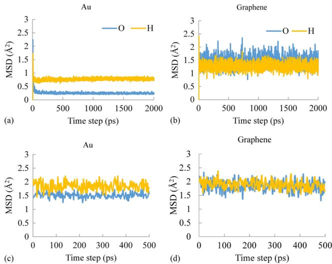
FIG. 10. Variation of MSD of hydrogen and oxygen atoms of water molecules at the interface of (a) Au (100) and (b) graphene. Variation of MSD of water molecules at the interface (blue) and adjacent layer (orange) of (c) Au (100) and (d) graphene systems.
