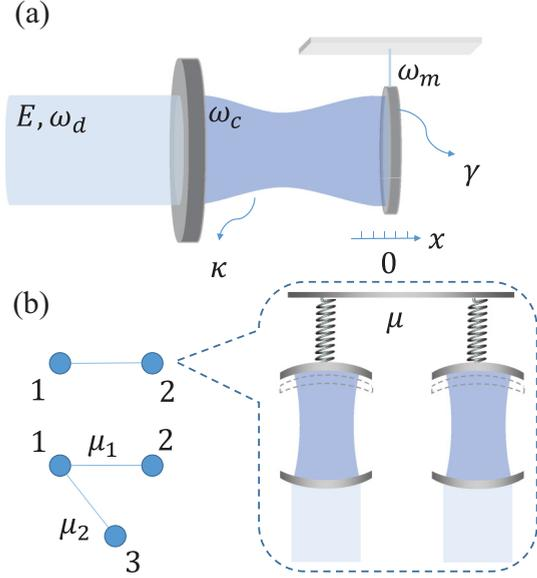
FIG. 1. (a) Schematic diagram of an optomechanical system: a mechanical resonator is coupled with a Fabry-Pérot cavity through the nonlinear radiation pressure force of a quantized optical mode. (b) Two kinds of coupling structures. Here, each node represents an optomechanical system, and the lines denote phonon tunnelings.
